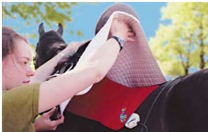
fixation of pliance horse sensor mat
